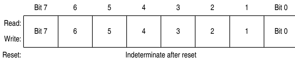
Figure 11-15. TIM Channel 1 Register Low (TCH1L)
