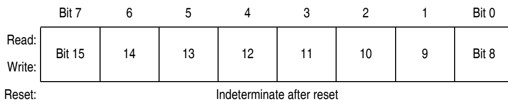
Figure 11-14. TIM Channel 1 Register High (TCH1H)
